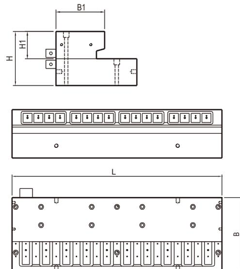
● Rail milling magnetic clamping system
